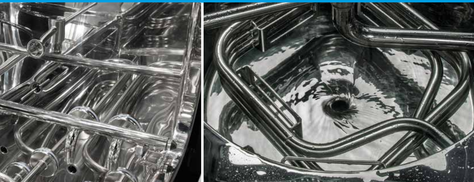
AISI 316L (1.4404) MIRROR FINISHING WITH ROUNDED CORNERS • PERFECT DRAINING OF TANKS AND LINES
